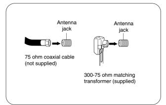
Connect the 75 ohm cable from the combination VHF/UHF antenna to the antenna jack on the back of the TV/DVD.
